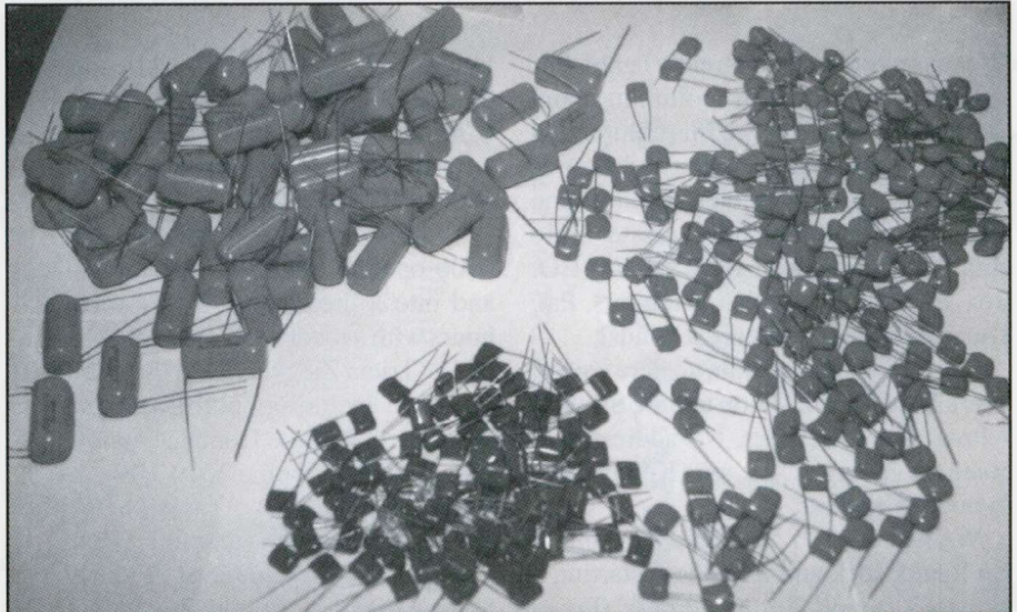
A recent order from Hosfelt arrives. Going clockwise from upper left: Sprague .22 mFd Orange Drops, .01 mFd Orange Drop style caps (not Sprague) and some .047 mFd capacitors.
